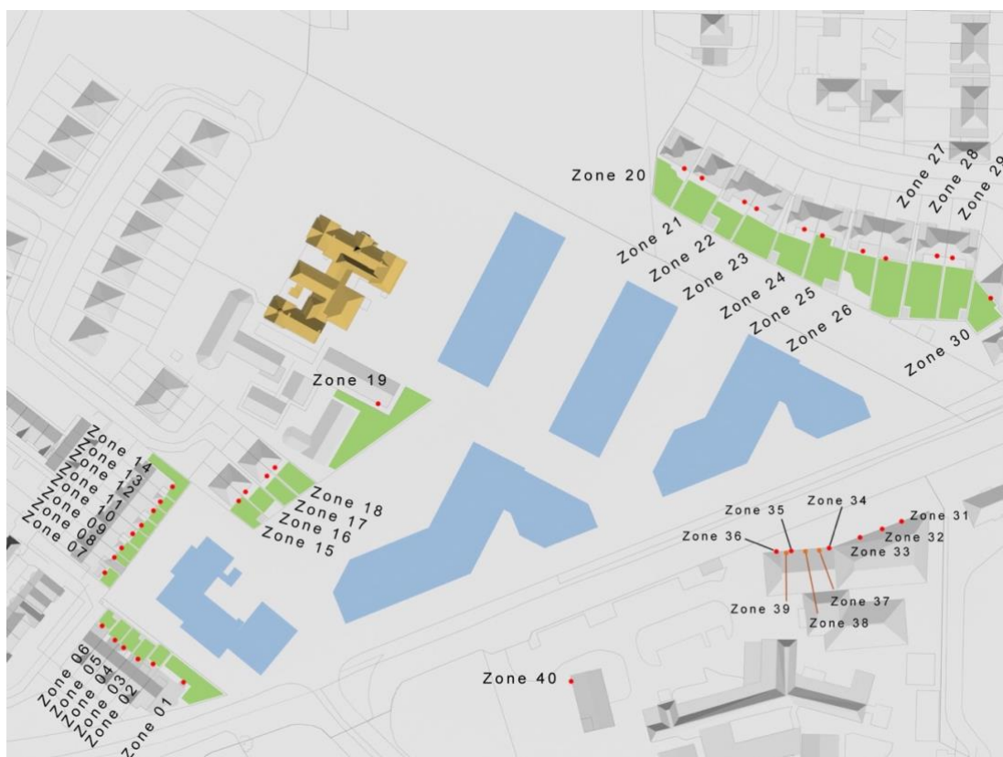
Figure 5.2 - Indicative diagram showing location of sample windows (indicated with red dot) and gardens (indicated in green) assessed under this chapter.
