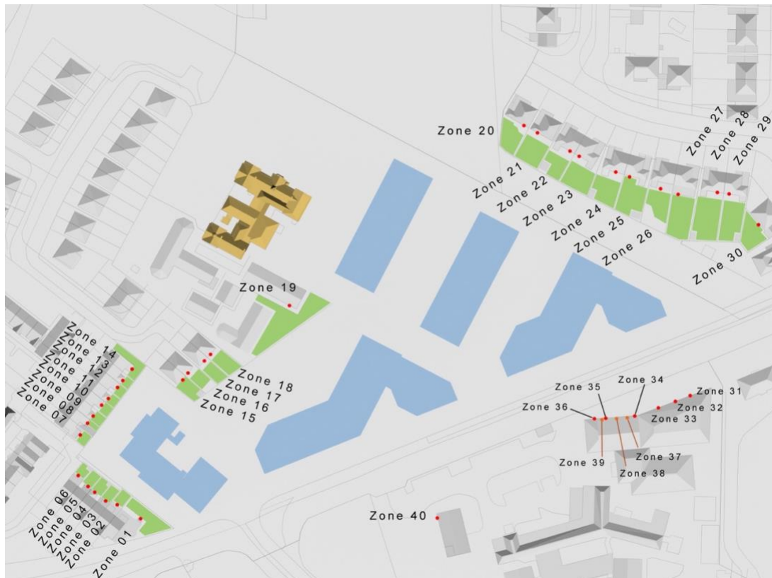
Figure 5.1 - Indicative diagram showing location of sample windows (indicated with a red dot) assessed under this chapter
