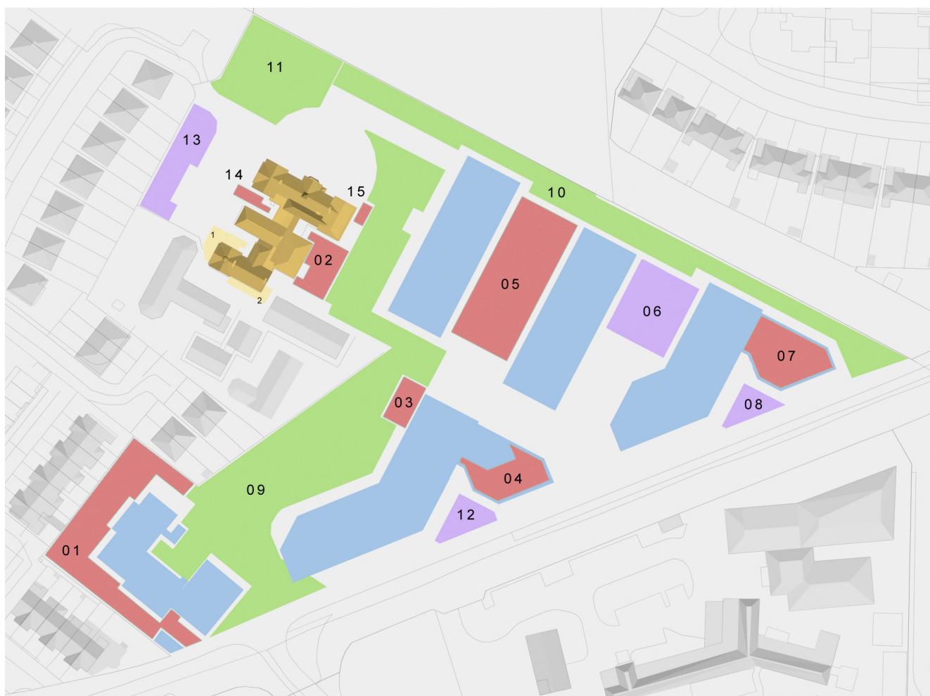
Figure 1 Indicative diagram showing location of open spaces within the proposed development assessed as part of this analysis. Communal open spaces are shown in red (Open Spaces 01, 02, 03, 04, 05, 07, 14 and 15). Public open spaces are shown in green (Open Spaces 09, 10, 11). Visual Amenity Open Spaces are shown in purple (Open Spaces 06, 08, 12 and 13). Creche Open Spaces are shown in yellow (Creche Open Spaces 1 and 2).
