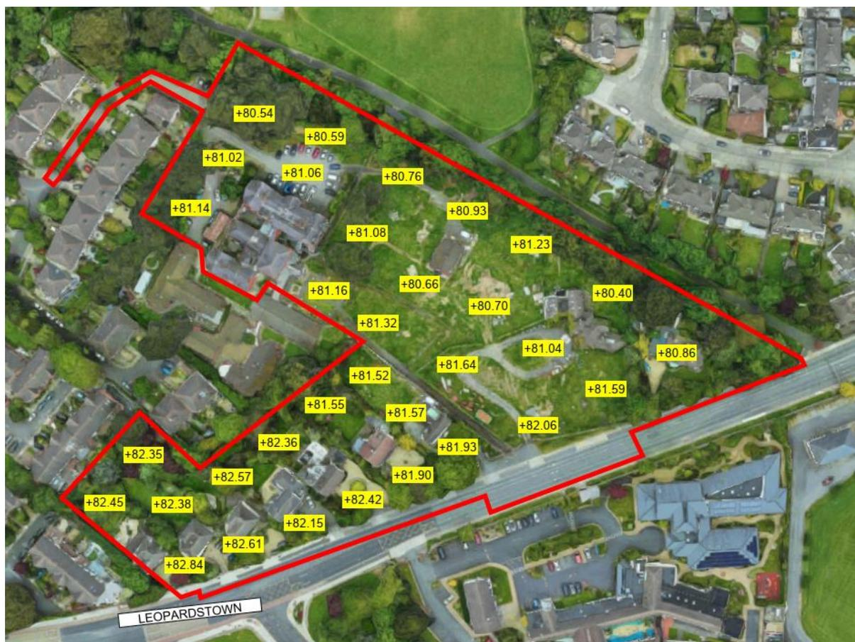
Figure 8-1 – Topographical Survey Extract
