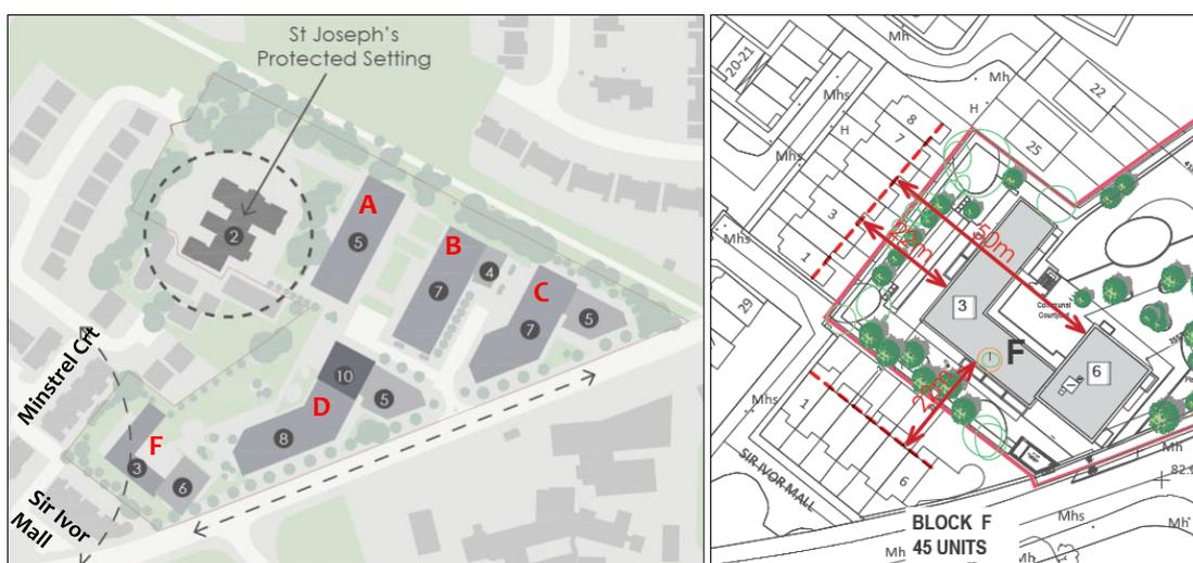
Figure 12.17 A & B Proposed Site Layout And Building Heights
