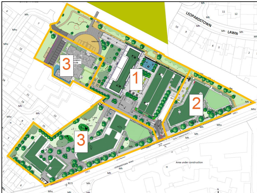
Figure 3.1 Site construction phasing strategy
